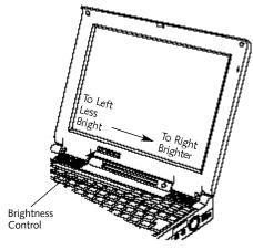
Figure 2-2 Display Adjustments
